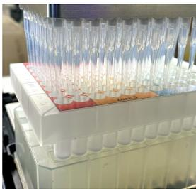
The resin was screened as a 200 µL slurry in triplicate for each sequence in a 96 well plate on the Beckman Coulter Biomek™ i7 liquid handling platform.
